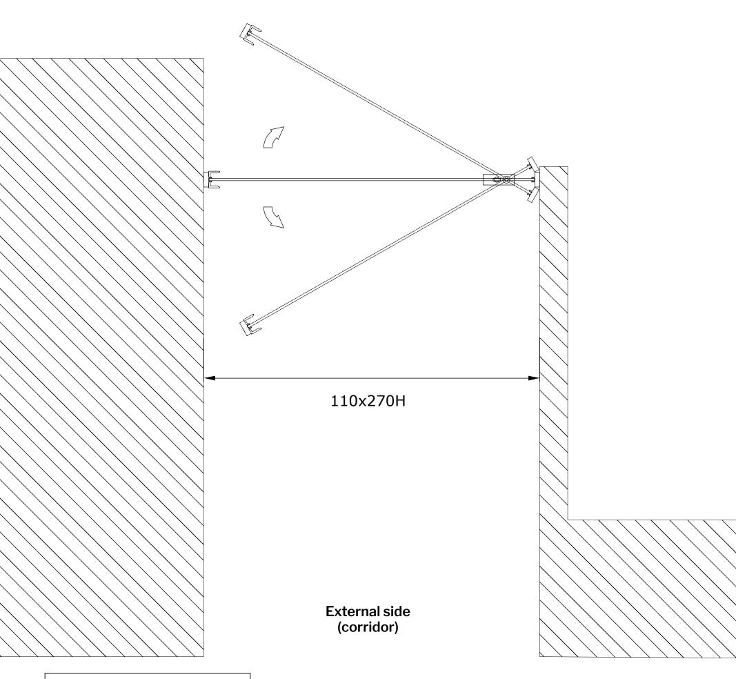
Floor plan layout of T-ES Design 24, single pivot door
