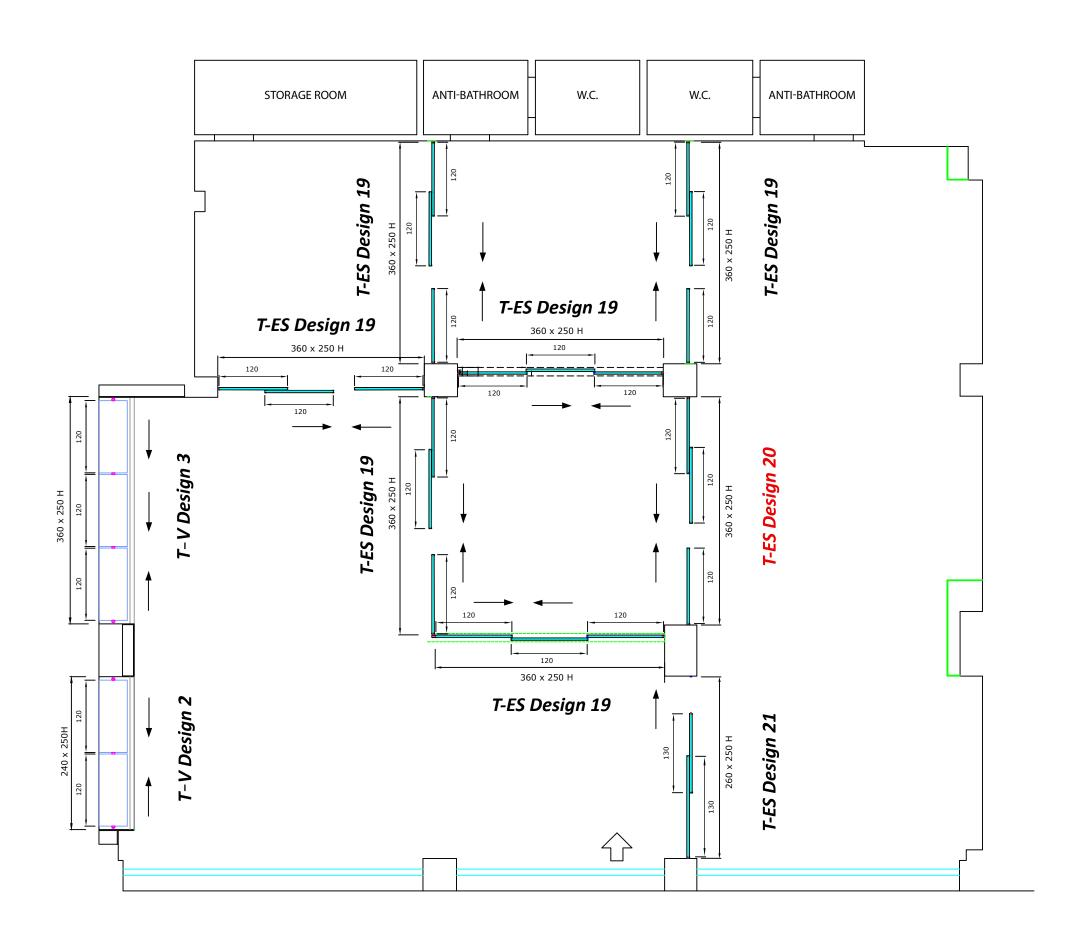
Plan layout of partition walls with sliding door openings.
