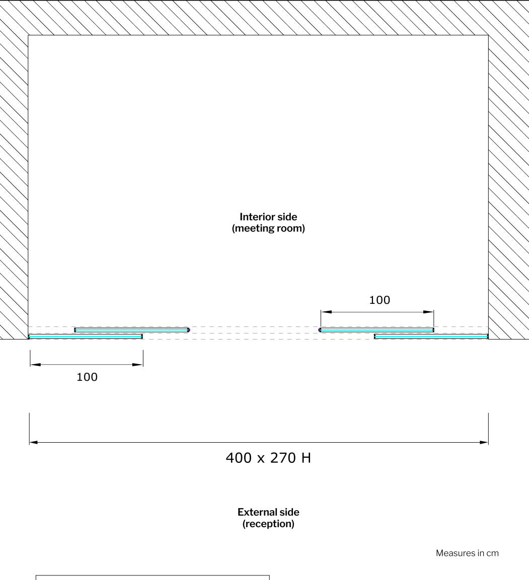
Floor plan layout of the T-ES Design 11, external sliding wall door with 4 symmetrical doors
